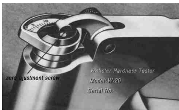
Fig.3 Regulate the adjusting screw
