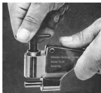
Fig.4 Regulate the adjusting nut
