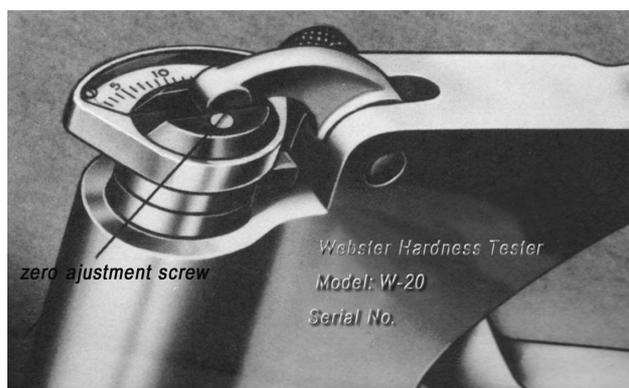
Fig.3 Regulate the adjusting screw
